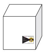
If the package is twice as long as it is wide, use two ShockDot impact indicators. Place a second indicator in the same position on the opposite side of the package.
